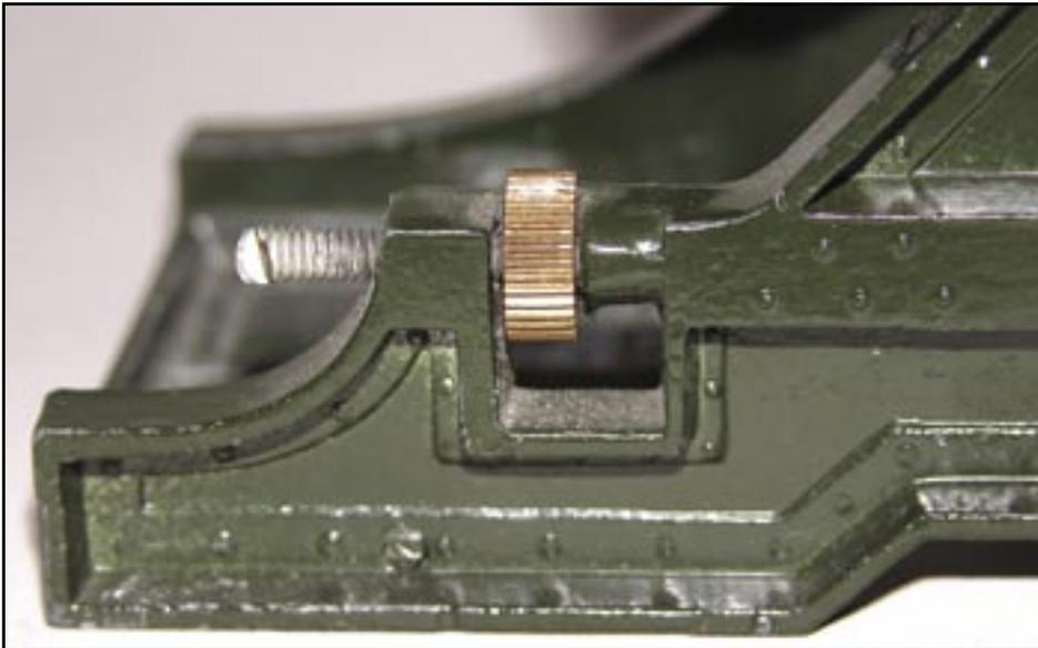
So the substitution of lead for brass as a suitable metal replacement in the production of the rotating elevation wheel does not seem to have made too much sense.
