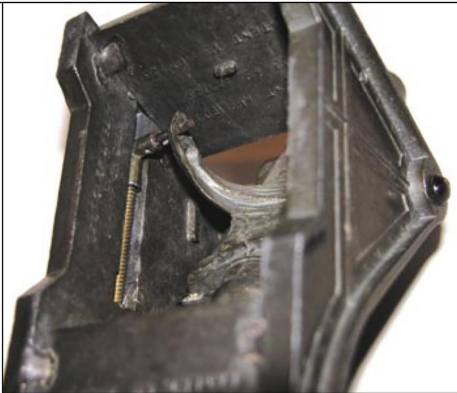
In any case, the complicated right angle knob was replaced by 1920 with a brass elevating rod with the end attached to the barrel formed by bending the rod at a right angle, leaving a tip about a half-inch long. All subsequent models had a bent rod connecting the barrel to the rotating wheel.
